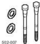
Subframe Alignment Bolt 502-007
